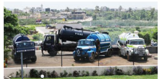
*Pump trucks dumping sludge at the adjacent fecal sludge treatment plant that now operates in conjunction with the OP*
