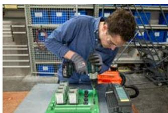
**Constructing one of the boiler control panels**
