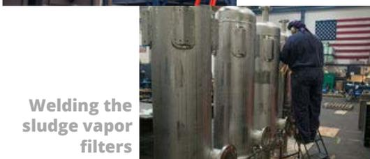
**Welding the sludge vapor filters**
